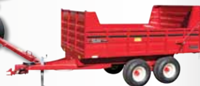
Dirt Boss Dumper 12 ton | 7' x 12' deck | 24" sides
